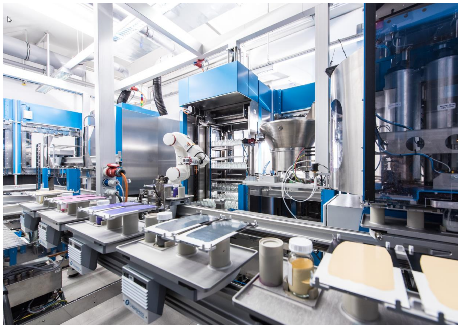
Caption: The new high-throughput plant in Essen can formulate and test up to 120 samples daily.
